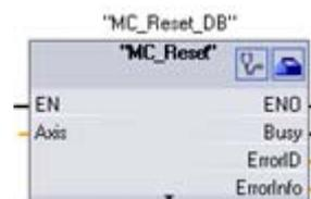
MC\_Reset resets all motion control errors. All motion control errors that can be acknowledged are acknowledged.
