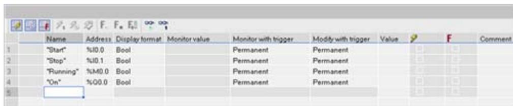
The various functions can be selected using the buttons at the top of the watch table.
