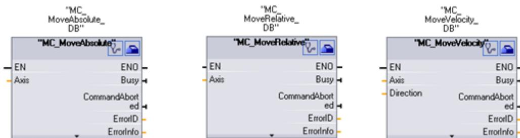
MC\_MoveAbsolute starts motion to an absolute position. The job ends when the target position is reached.
