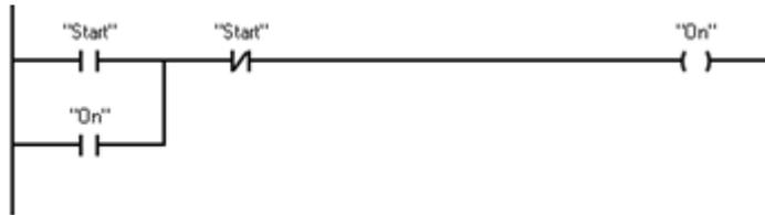
The elements of a circuit diagram, such as normally closed and normally open contacts, and coils are linked to form networks.
