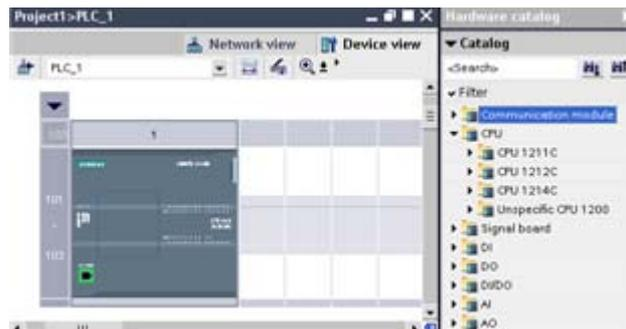
Selecting the CPU in the Device view displays the CPU properties in the inspector window.
