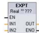
Click below the box name and select a data type from the drop-down menu. EXPT parameters IN1 and OUT are always Real. You can select the data type for the exponent parameter IN2.
