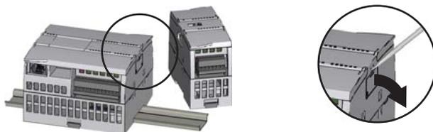
Remove the cover for the connector from the right side of the CPU.
