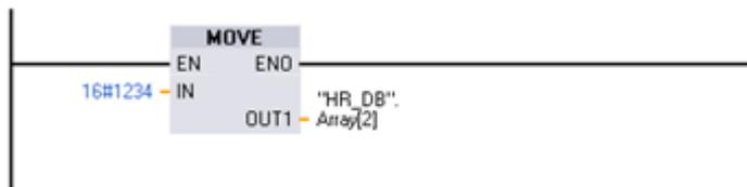
Each of the words in the array, as defined in the data block, provides the MB\_SLAVE instruction with Modbus holding register addresses. In this instance, since there are only 10 elements in the array, there are only 10 available Modbus holding register addresses usable by this MB\_SLAVE instruction and accessible by a Modbus master.
