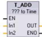
Select the IN1 data type from the drop-down list available below the instruction name. The IN1 data type selection also sets the data type of parameter OUT.
