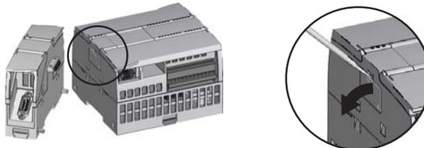
Remove the bus cover. Retain the cover for reuse.
