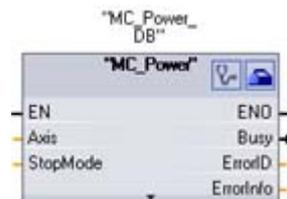
MC\_Power enables and disables a motion control axis.
