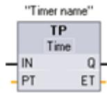
TP, TON, and TOF timers have the same input and output parameters.
